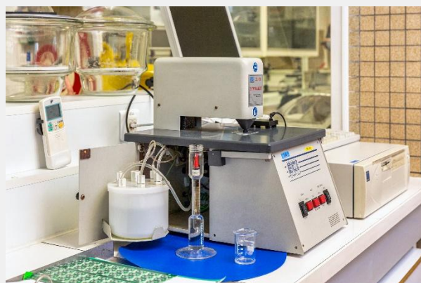
> SERA Pure Tin plating thickness evaluation
