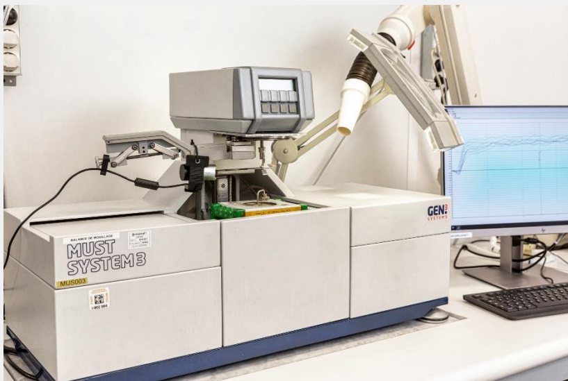
> WETTING BALANCE (MUST SYSTEM III) Solderability test
